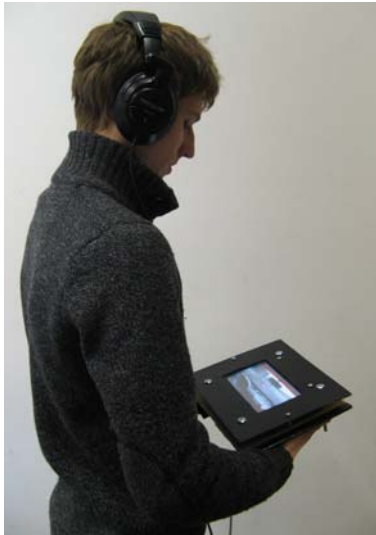
Figure 1: Prototype UltraTV concept. The user hears, sees and feels the content in the video stream.
