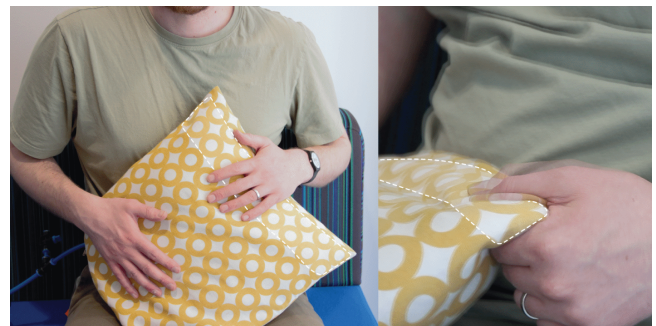
Figure 19: Interactive Force-Feedback Cushion, that enables tactile input and feedback using a soft deformable pouch, without compromising the cushion’s original softness. The white dashed line indicates the outline of the embedded TPU pouch
