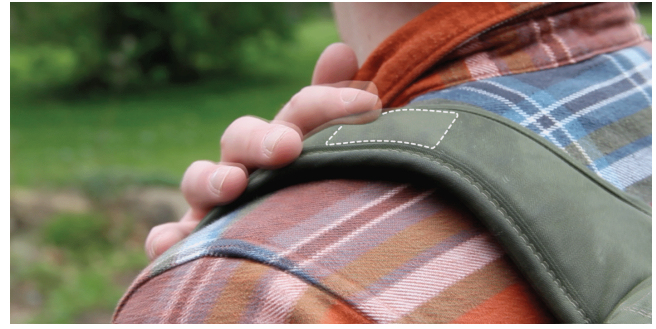
Figure 18: The “Wayfinding” Force-augmented Backpack provides tactile on-body feedback from force applied through a backpack strap, facilitating spatial and temporal notifications while integrating into an existing backpack. The white dashed line indicates the outline of the embedded TPU pouch.
