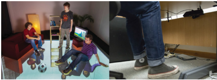
Fig. 4. Extrinsic sensing from below with an FTIR floor [Bränzel et al. 2013] and from above with a Kinect sensor [Simeone et al. 2014].
