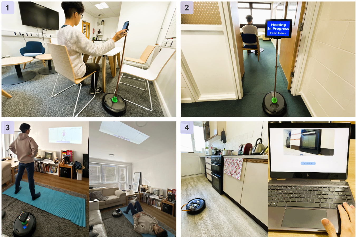
Figure 16: Implemented Applications: (1) The robot serves as a mobile wireless charger. The robot follows the user, and the user can charge the phone by placing it in the holder, (2) The robot shows the user's busy status using the attached screen, (3) The robot projects a workout video on the wall (Left) and on the ceiling (Right), (4) The user monitors the home remotely and has task control of the home with live video. The robot observes the oven (Left), and the user watches the live video and controls the robot (Right).
